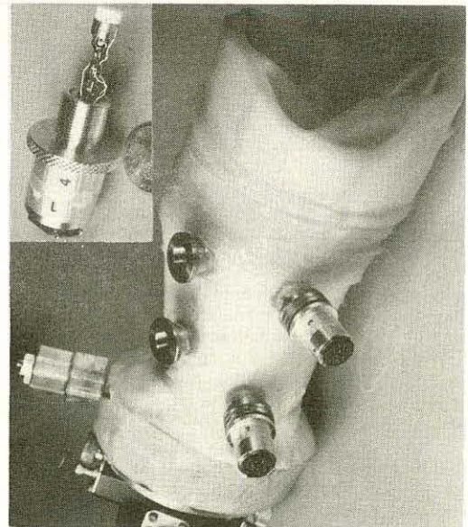
FIGURE 1: An instrumented socket with transducers positioned in two of four anterior measurement sites. (cable not shown). Inset: transducer close-up view.
