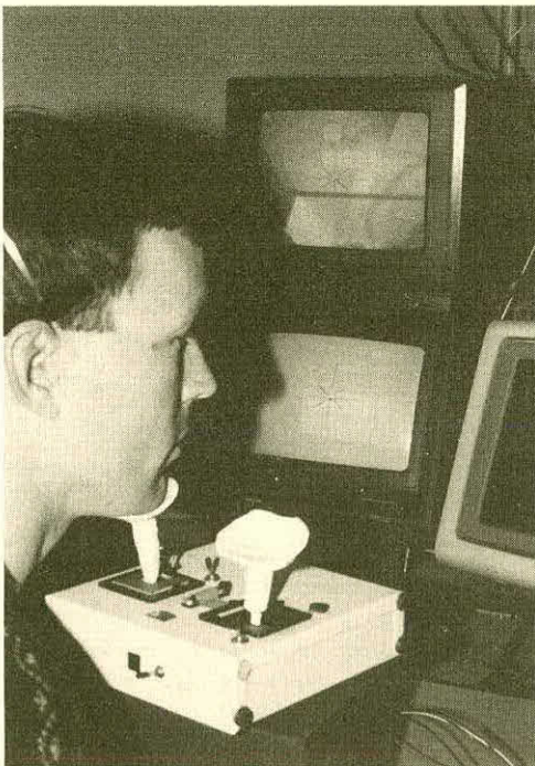
Operating a workspace-mouse: a triangulation algorithm locates an object when remote control camera crosshairs are aligned.
